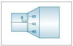
The pitch of the screw = 1 mm L.C. of screw gauge = 0.01 mm Main scale reading = 2.5 mm 46th division of circular scale coincides with the base line. Therefore, circular scale reading =  $46 \times 0.01 = 0.46$  mm Total reading = Main scale reading + circular scale reading = (2.5 + 0.46) mm = 2.96 mm
