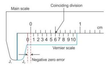
To find this error, we note the division of the vernier scale coinciding with any division of the main scale. The number of this vernier division is subtracted from the total number of divisions on the vernier scale and then the difference is multiplied by the least count.
