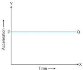
The area enclosed between the straight line and time axis for each interval of time gives the value of change in speed in that interval of time.
