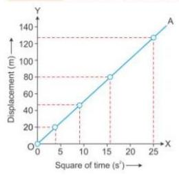
The value of acceleration due to gravity (g) can be obtained by doubling the slope of the  $S - t^2$  graph for a freely falling body.
