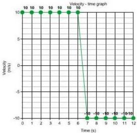
Distance travelled in first  $6 s = velocity \times time$
